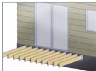
Joists securely attached for better safety
